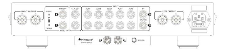
At the rear panel, you will find your inputs, eventually the HT Pass-Thru, the speaker terminals, Tape Out and Sub Out.
