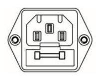
**Mains Fuse:** The Mains fuse is located on the amplifier's rear, just below the power cord socket (see picture on the left). The fuse rating is 1 x **Littelfuse 213 Series 6,30A** Slow Blow 5 x 20mm fuse for 100-125VAC and **Littelfuse 213 Series 3,15A** Slow Blow 5 x 20mm fuse for 200-250VAC.
