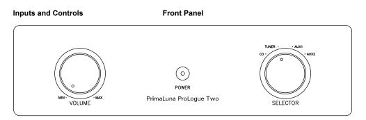
The front panel of the PrimaLuna models is made from machined aluminium, finished to match the blue metallic chassis. The volume is controlled with the knob on the left, source selection is on the right. Your sources are labelled CD, Tuner, Aux 1 and Aux 2, but all are interchangeable. There is no functional difference between the inputs. The power switch is located on the left side of the amp, just behind the front plate.
