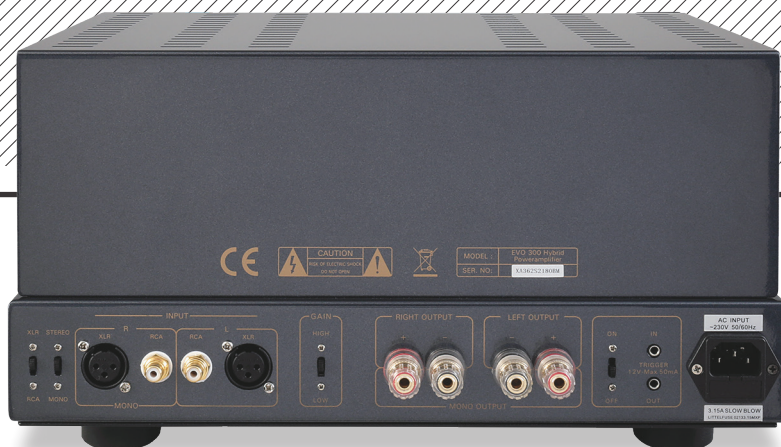
ABOVE: The EVO 300 Hybrid 'poweramp' differs from the 'integrated' with its bridge (mono) mode and balanced XLR input option. Overall gain is also switchable as are the 12V trigger ports. Speaker outs are on gold-plated 4mm cable binding posts
