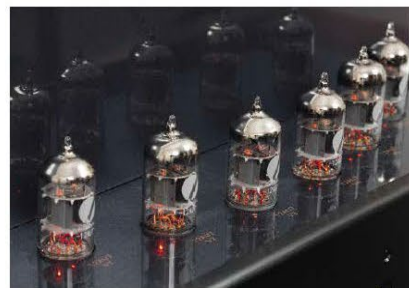
The preamp is tube-based, with six tubes at work.
