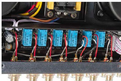
The input selection relays are just behind the RCA input sockets at the rear panel. The signals flow via long cables to the front panel.
