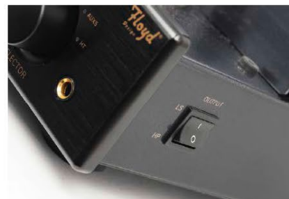
A similar switch on the other side serves as the output selector (speaker/headphone).
