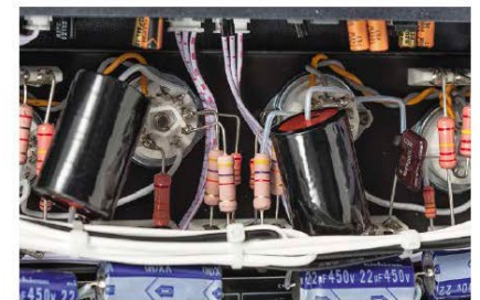
The connections are point-to-point wired in the area around the tubes. The remaining circuits are on printed circuit boards.
