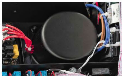
In the preamplifier section, there are two transformers.
