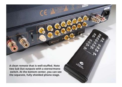
The amplifier has an input for using the output stage only but also dual subwoofer outputs. To maintain the sound character between the bass and the speakers, it has been decided to let the bass outputs be fed by the power stage via transformers, and not in the conventional way where you take the sub-signal from the line stage. An unusual solution, then, which PrimaLuna, like subwoofer manufacturer REL, believes not only provides better sound integrity but also greater dynamics.
