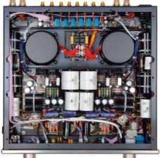
The input stage is on the bottom side with dual power supplies and transformers.Components are consistent with very high quality and at the forefront are the directly soldered tubes.
